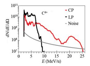
*Fig.2.* C<sup>6+</sup> spectra with vertical axis units of particles/MeV/sr for 10 nm amorphous carbon targets irradiated with CP (red) and LP (black) laser pulses.
