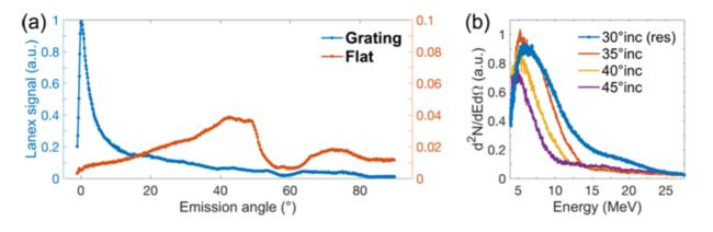
Figure 1(a): Electron spatial distribution from tangent (0°) to normal (90°) for flat and grating targets irradiated at 30°;
