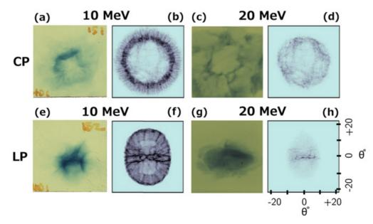
Fig.3. CP (a-d) and LP (e-h) proton beam profiles at 10 MeV (left) and 20 MeV (right) obtained experimentally from 10 nm amorphous carbon targets on RCF (a,c,e,g) and through 3D PIC simulations (b,d,f,h). All images represent the same solid angle of the beam profile (marked in h).
